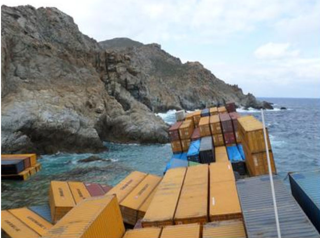
Figure 11: Yusuf Cepnioglu listed to portside with some containers toppled into the sea.
