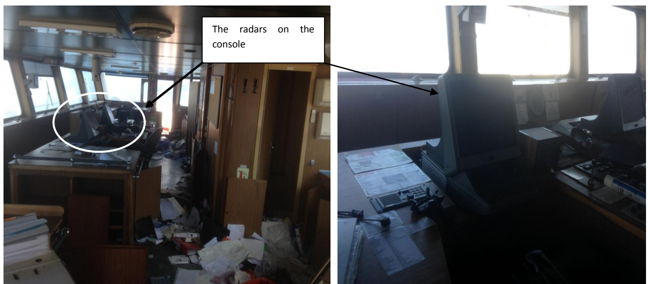
Figure 16: General view of the bridge arrangement and the two radars at the main console
